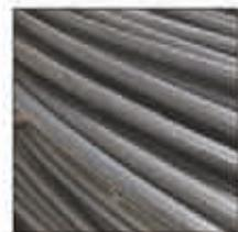
Hot and cold coiling technology is used to produce KYB K-Flex springs. A carefully controlled shot-peening process significantly increases the fatigue life of the coil spring. All K-Flex coil springs are phosphate coated prior to receiving an epoxy powder coating. This process guarantees a tough, durable finish with enhanced corrosion resistance properties.
